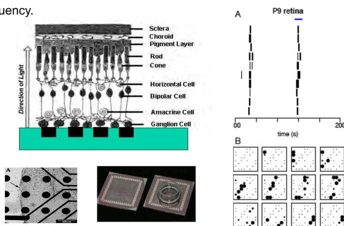
**Figure 1:** Diagram of retina on MEA. Most of the data is acquired from a 8 x 8 (without the 4 corners) grid of electrodes (30  $\mu\text{m}$  across, 200  $\mu\text{m}$  apart), acquired at 25 kHz. Local field potentials as well as individual spike times are typically recorded. We extract spike times and record activity bursts/waves across the array.
